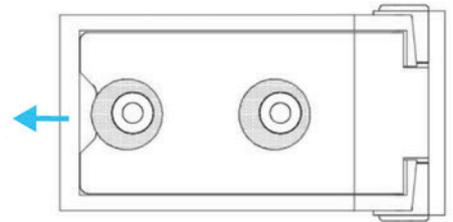
to adjust the hinges, rotate the think parts and make sure the final position is as shown as illustrated.
