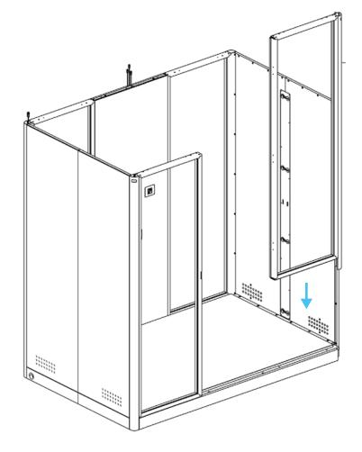
Hold the glass frame on a higher level of the wall panel, put it against the wall and slide it into the floor.
