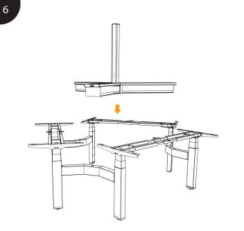
Finally attach the accesories on top of the standard Matrix Pro Wing.
