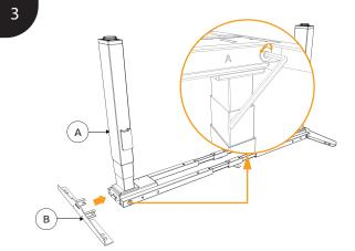
Attach B to A by secure the pre-assembled screw using Allen key.
