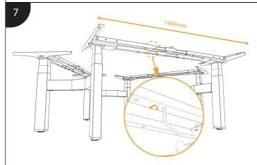
Adjust the table length to 1480mm and secure the screw using Allen key. Repeat this step on the other 2 remaining legs.
