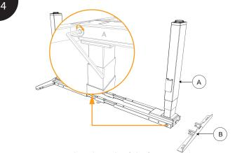
Repeat Step 3 on the other side of the frame A and repeat it 4x to the rest of Part A and B.
