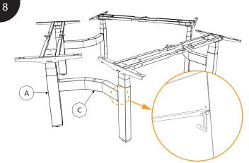
Finally secure the lock plate under the C with screw using Allen key. Repeat this step 2x to the other part of the legs.
