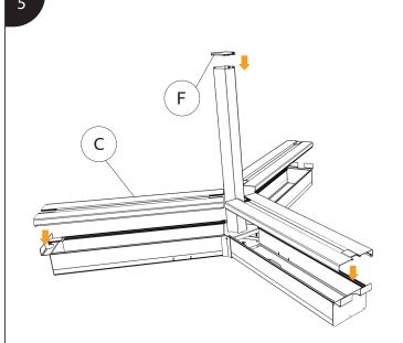
Cover up both part with C and F. Repeat this step 2x for Component C.
