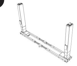
Raise the legs, slide the frame outwards to fit desired size and fix it with the bolts that are already mounted in the frame.
