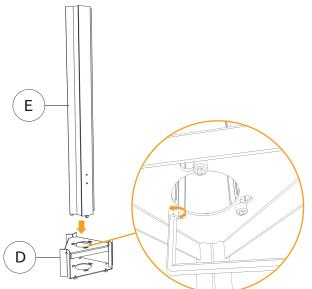
Attach E (with the pre-install screw) to the key hole of D and tighten it using Allen key.
