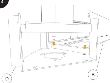
Screw B to D by using JCBC screw. Repeat this step for another 2x to the rest of the components.
