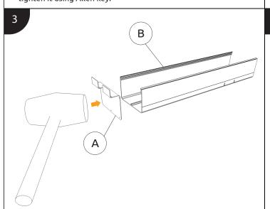
Use Mallet to attach A to B. Repeat this step for another 2x to the rest of the components.
