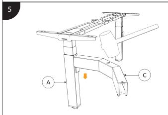
Attach C to A by using mallet.
