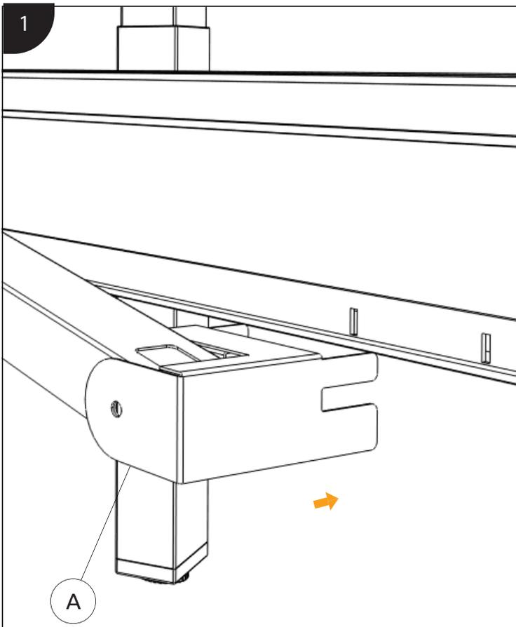
Attach A by slotting it's bottom adapter into the Main Gutter holes.
