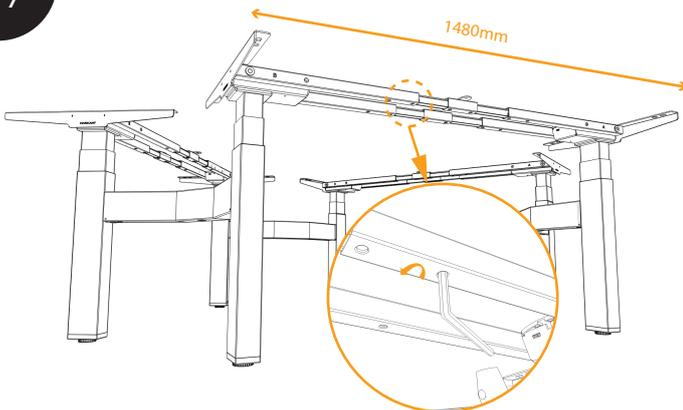
Adjust the table length to 1480mm and secure the screw using Allen key. Repeat this step on the other 2 remaining legs.
