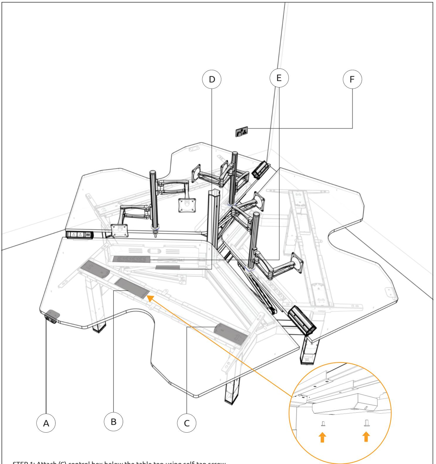
STEP 1: Attach (C) control box below the table top using self-tap screw.
