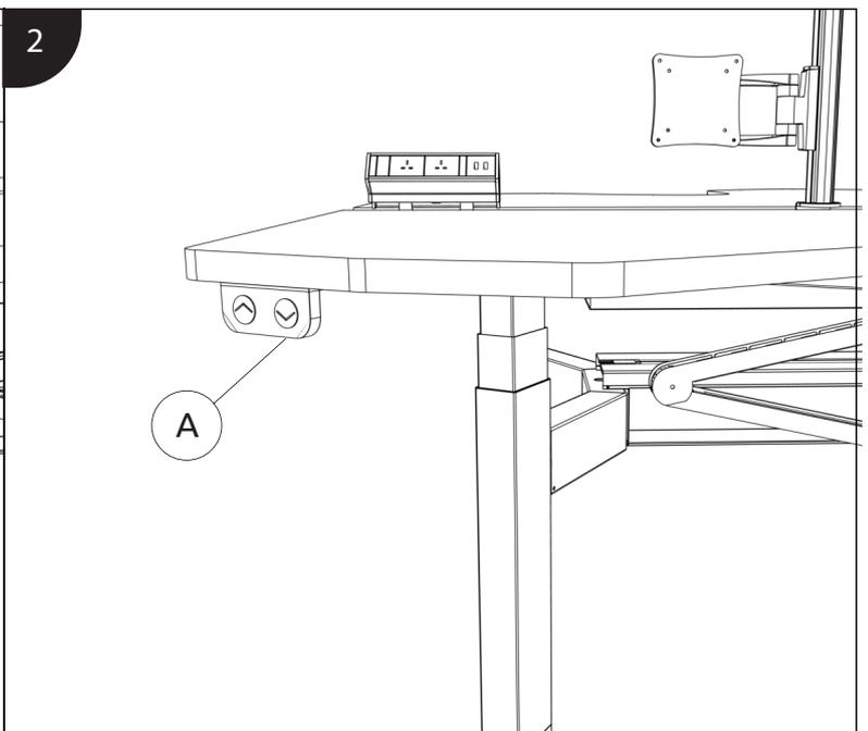
The installation for (A) Handset is completed.
