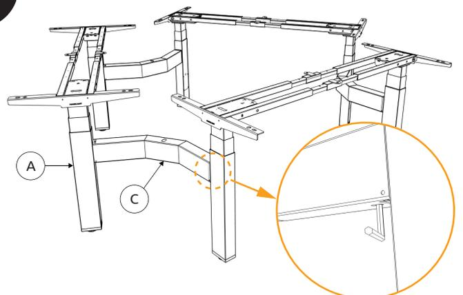
Finally secure the lock plate under the C with screw using Allen key. Repeat this step 2x to the other part of the legs.
