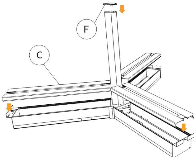
Cover up both part with C and F. Repeat this step 2x for Component C.
