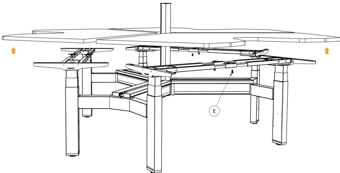
Attach table top on the frame and secure it using (E) screw. Repeat this step 2x on the other frame.
