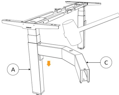
Attach C to A by using mallet.
