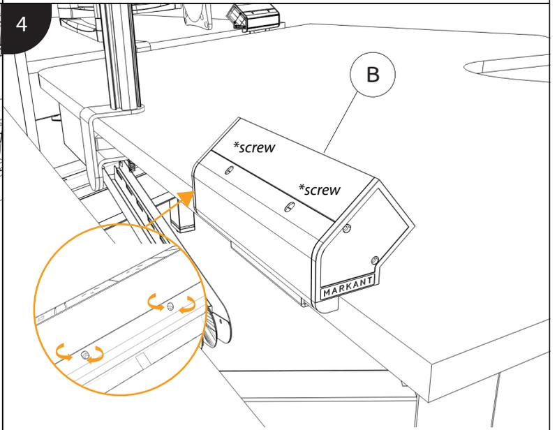
Tighten the screw on top of (B) Media Hub. The installation for Media Hub is completed.
