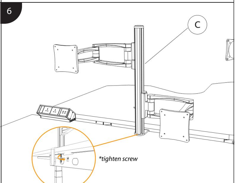
Tighten the screw at the bottom. The installation for (C) Monitor Arm is completed.
