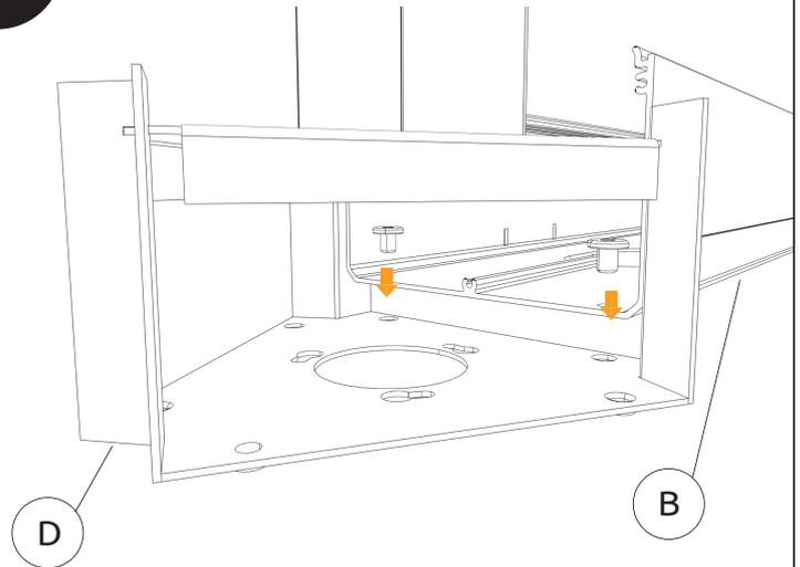
Screw B to D by using JCBC screw. Repeat this step for another 2x to the rest of the components.
