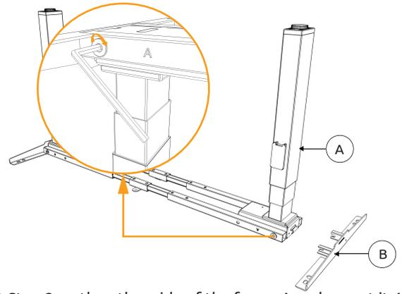
Repeat Step 3 on the other side of the frame A and repeat it 4x to the rest of Part A and B.
