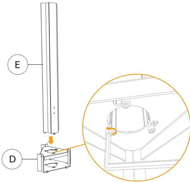
Attach E (with the pre-install screw) to the key hole of D and tighten it using Allen key.
