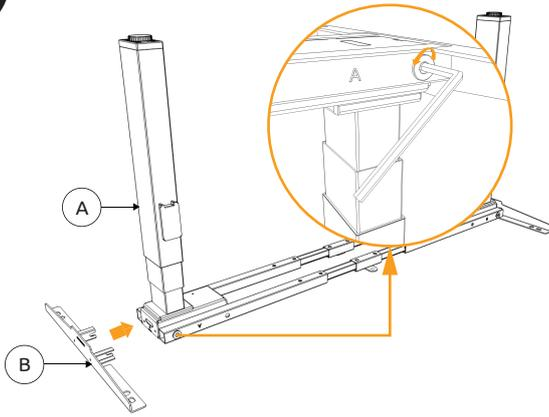
Attach B to A by secure the pre-assembled screw using Allen key.
