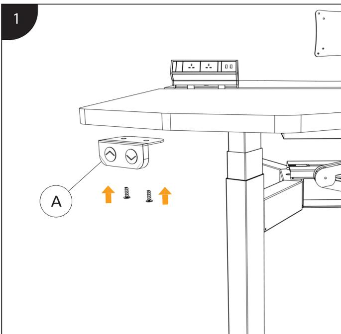
Attach (A) Handset below the table top using a screw.
