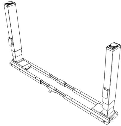
Raise the legs, slide the frame outwards to fit desired size and fix it with the bolts that are already mounted in the frame.
