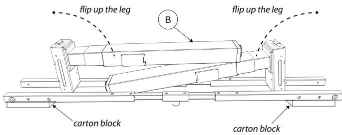
The frame (B) is pre-assembled. Do not remove the carton box until the leg is flip up. This is to prevent any further damages.
