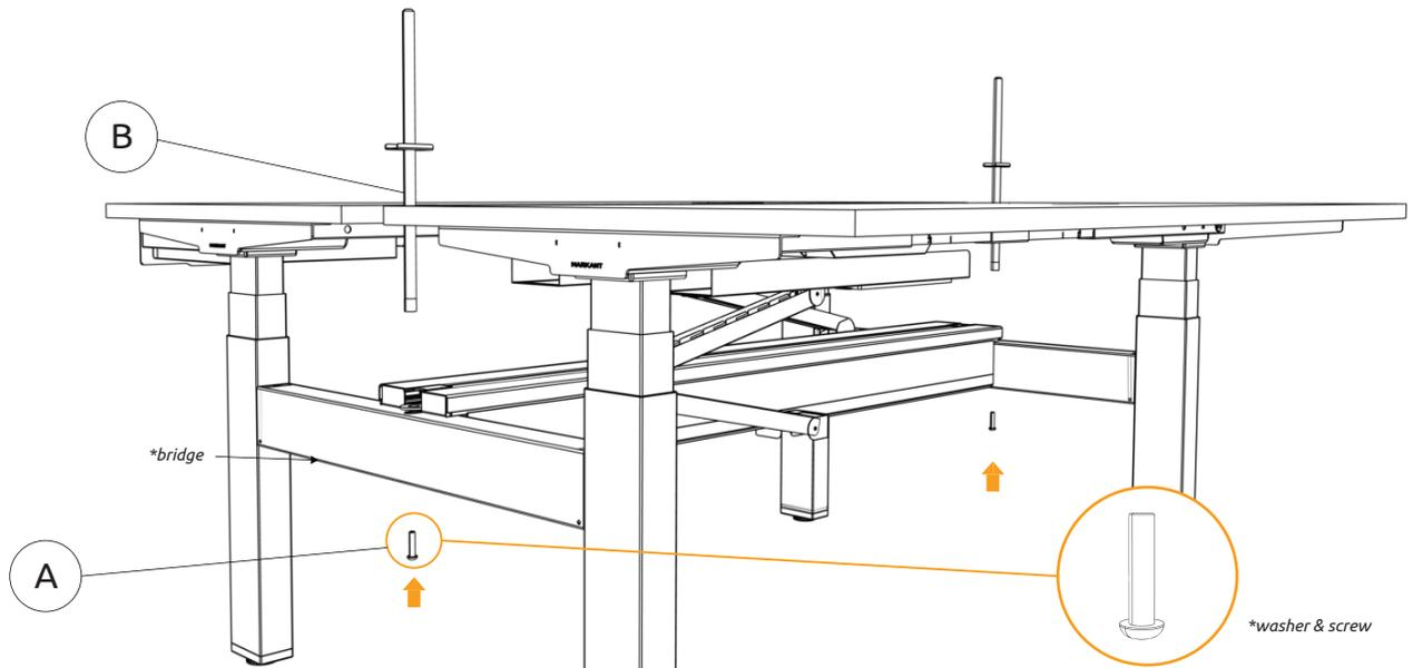
Slot in A into the bridge's holes. Secure it's position by tighten it to B with washers and screws as provided.
