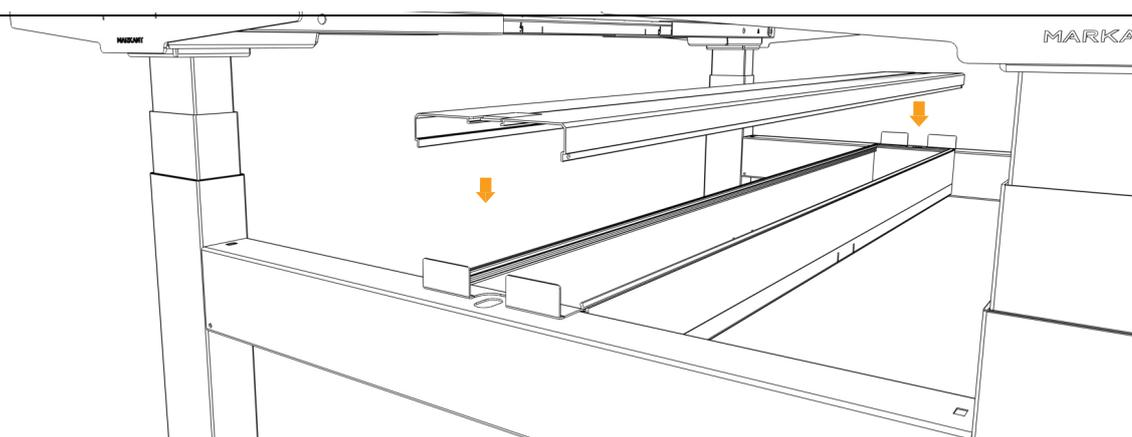
Finally, place the lid on top of the Main Gutter.
