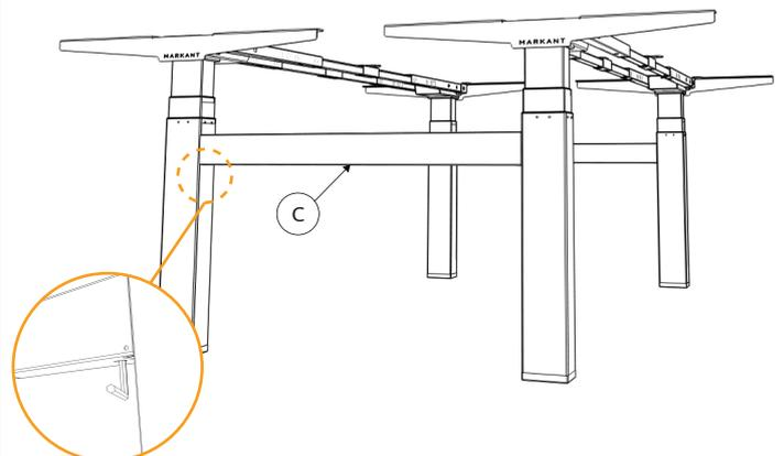
Finally, secure the lock plate under the C with screw using Allen key. Repeat this step to the other part of the leg.
