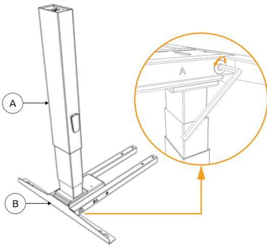
Attach B to A and secure the screw using Allen key. Repeat this step on the other side of the leg.
