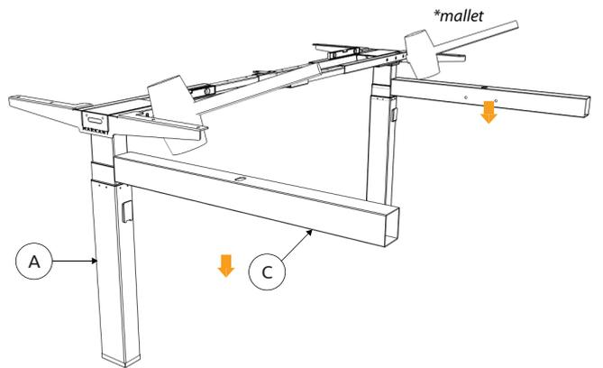
Attach C to A by using mallet. Repeat this step on the other side of the leg.
