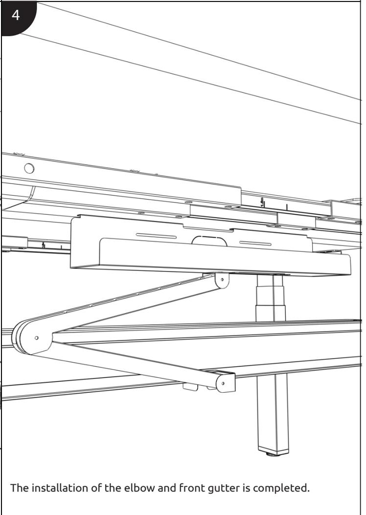
The installation of the elbow and front gutter is completed.
