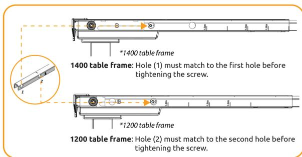
Adjust the table length and secure the pre-installed screw using Allen key.
