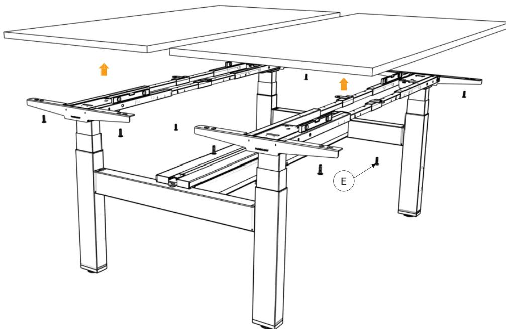
Attach table top on the frame and secure it using (E) screw.
