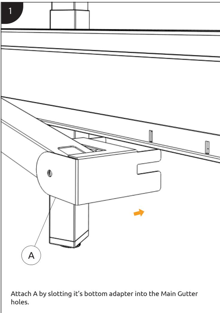
Attach A by slotting it's bottom adapter into the Main Gutter holes.
