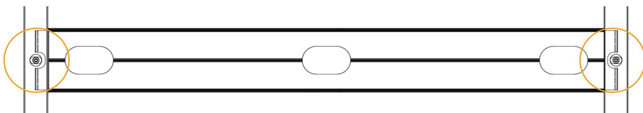
Make sure the cutout of the Side Covers is positioned at the center with the holes of the C brackets.
