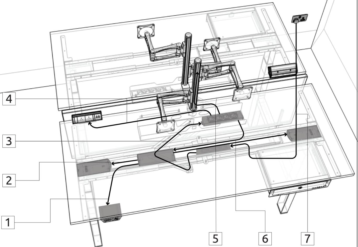
STEP 3: Attach the cable point to the rest of the accessories.
