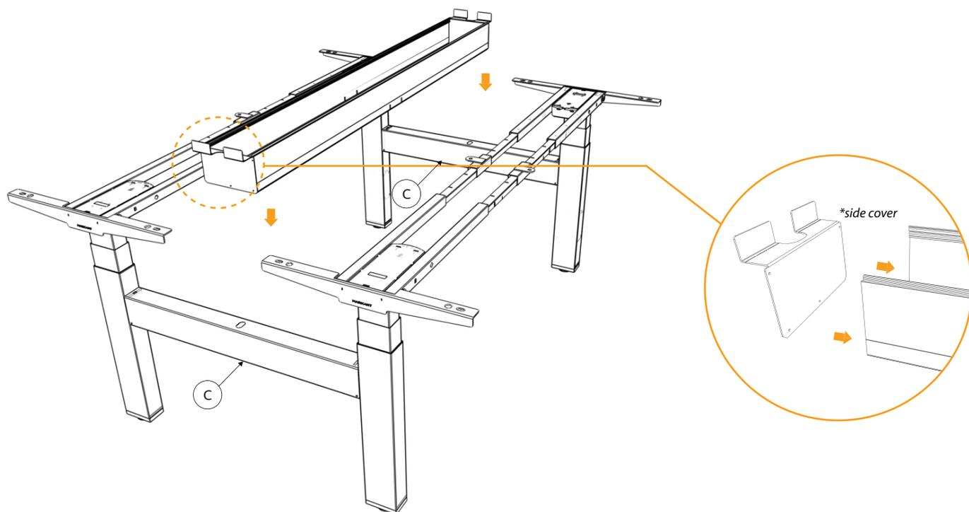
Place the Main Gutter in between the C. Prior to that, the Main Gutter need to be install with its Side Covers to make sure it is placed properly on the brackets. This can be done by hammer it using rubber hammer (i.e Mallet) to secure its position.
