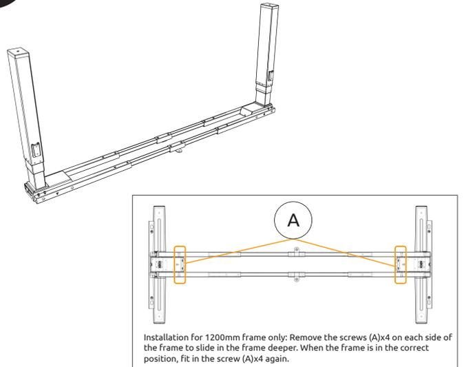
Installation for 1200mm frame only: Remove the screws (A)x4 on each side of the frame to slide in the frame deeper. When the frame is in the correct position, fit in the screw (A)x4 again.
