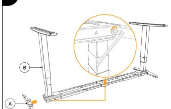
Attach A to B and secure the screw using Allen key. Repeat this step on the other side of the leg.
