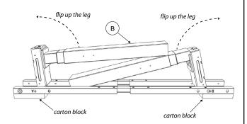
The frame (B) is pre-assembled. Do not remove the carton box until the leg is flip up. This is to prevent any further damages.
