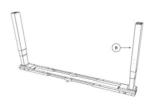
Raise the legs, slide the frame outwards to fit desired size and fix it with the screw that are already pre-mounted in the frame.
