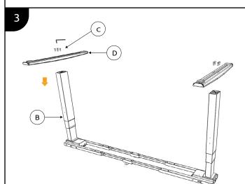
Attach D to B and tighten it with screw (C) using Allen key. Repeat this step on the other side of the leg.
